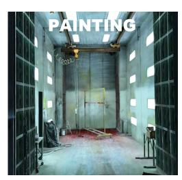
Our 15' x 30' paint booth can accommodate large or multiple small projects. With its high capacity air take-up unit and temperature control system, a custom quality paint finish can be applied year round.
